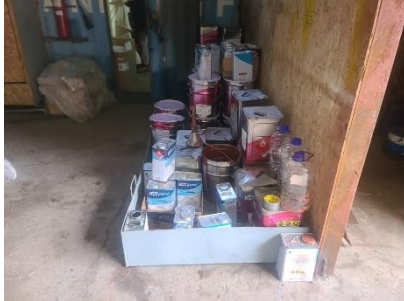
Figure 26. Secondary containment of chemicals at storage area of CC ZMEC (Status in January 2023)
